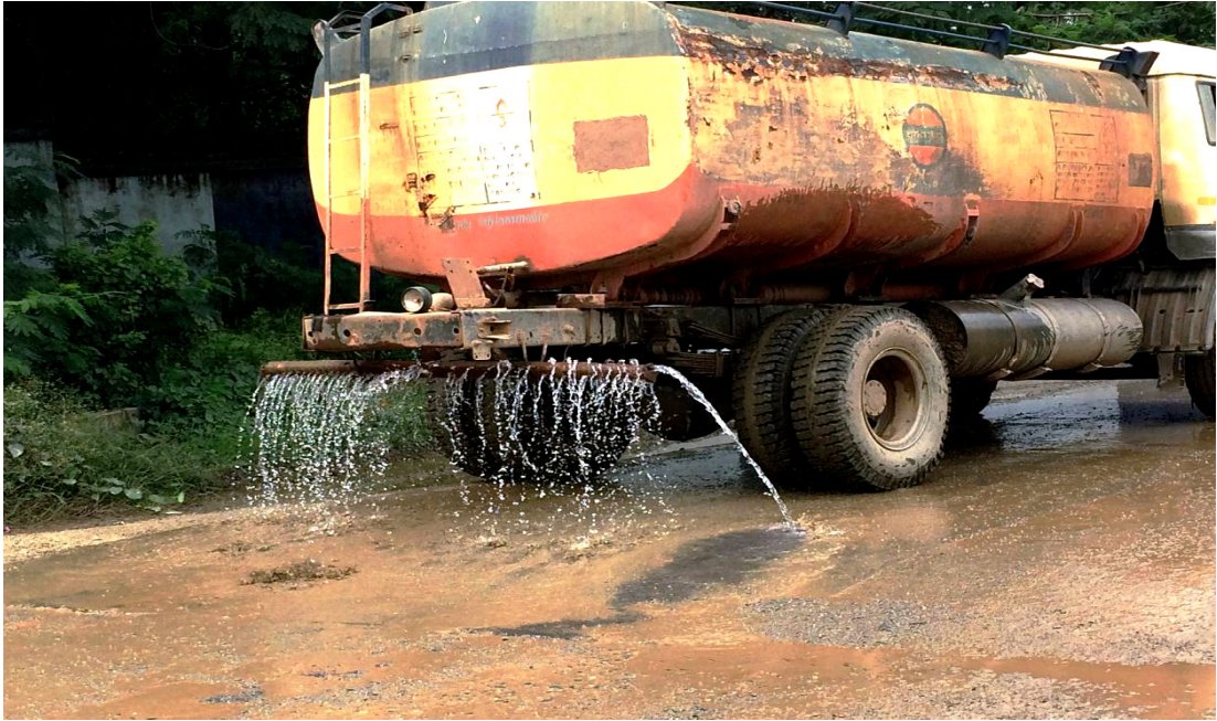
Photograph showing water sprinkling in haul road
